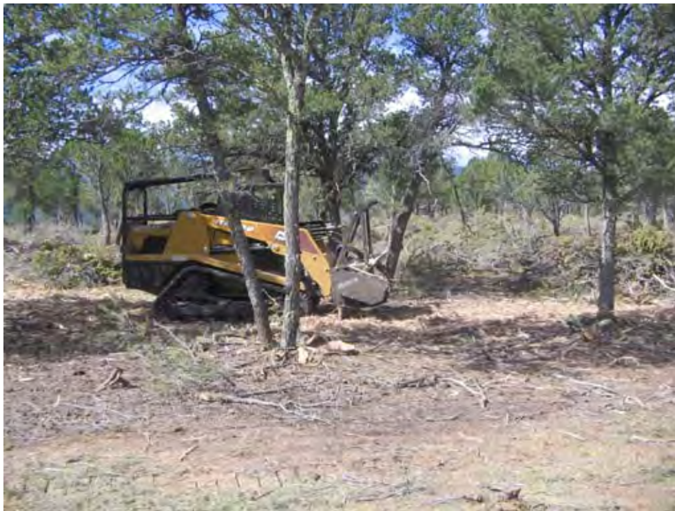
Figure 8. Thinning using a masticator.
